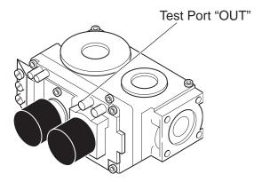
Figure 16 - Pressure Test Point Location
